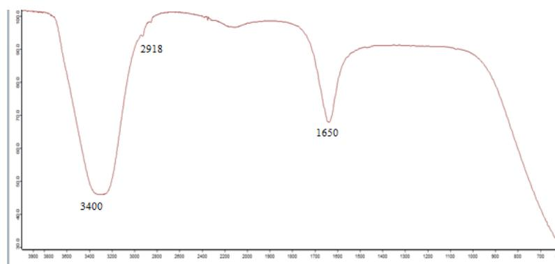
**Figure 2.** Attenuated total reflectance Fourier transform infrared spectroscopy (ATR-FTIR) analysis of silver nanoparticles (AgNPs). A portion of the synthesized AgNPs was analyzed using ATR-IR. The result showed the presence of absorption bands at 3400, 2918, and 1650 cm<sup>-1</sup>, which suggested the presence of a C-H bond, C-N and C-C bonds and N-H and C-N bonds, respectively.
