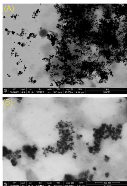
**Figure 3.** Transmission electron microscope (TEM) micrograph of silver nanoparticles (AgNPs). (A: 1 µm and B: 200 nm). A portion of the synthesized AgNPs was analyzed using TEM. The results showed that AgNPs were spherical in shape and polydispersed, but most of their sizes ranged from 10 to 35 nm.
